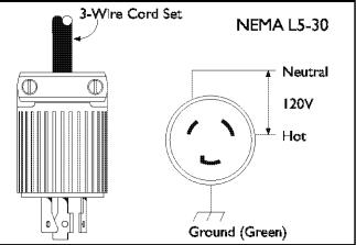
Use this receptacle to operate 120 Volt AC, 60 Hz, single phase loads requiring up to 3,600 watts (3.6 kW) of power at 30 Amps. The outlet is protected by a 30 Amp push-to-reset circuit breaker.
